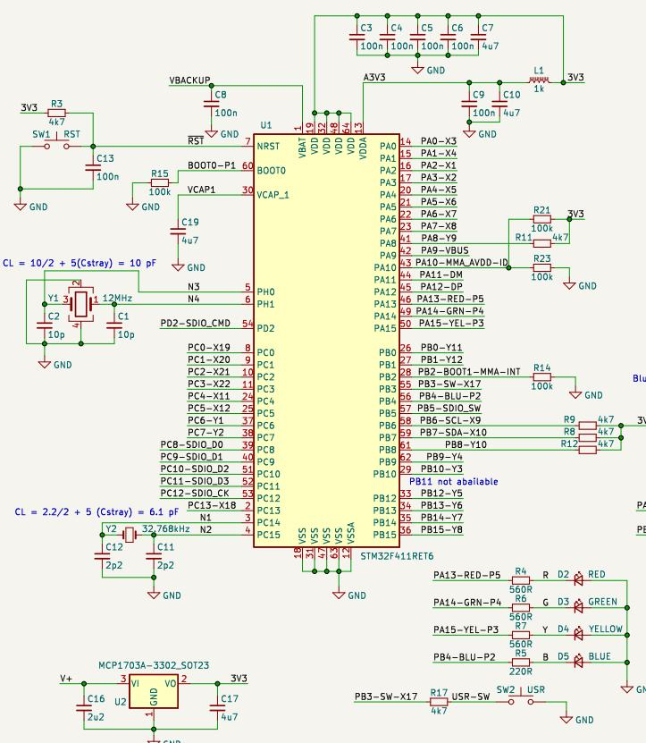
USB DFU requires stable levels on PA10, PB5, PB11 & PC11. PB2 must be low during boot. R12, R13, R20, & R21 provide stable input levels for DFU.
